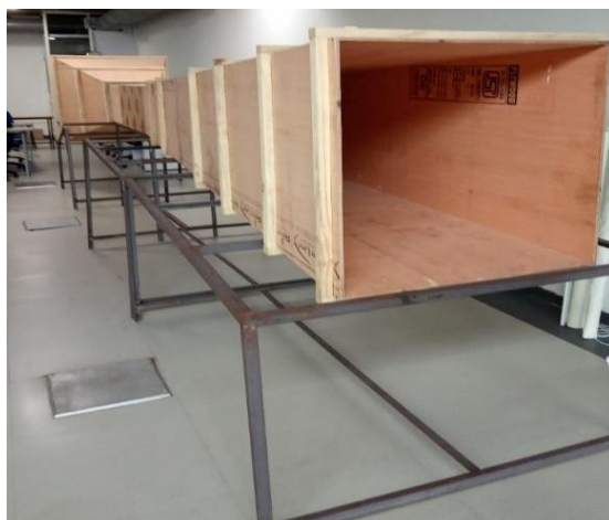
Fabricated 30 ft length Wooden Wind Tunnel
